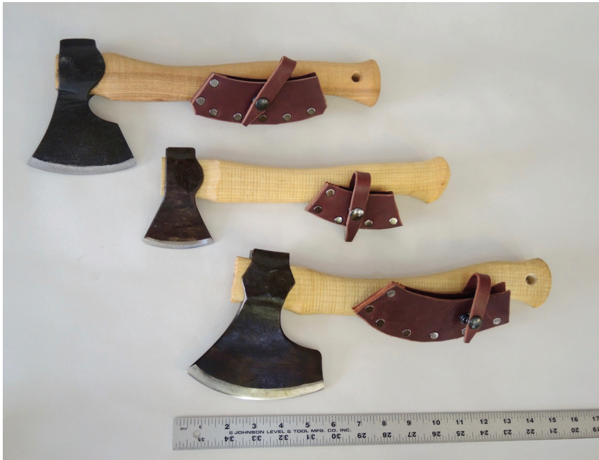
This is my favorite broad axe, used to hew most of the logs for our house. The hickory handle is bent away from the blade, to give clearance for your hands passing the hewed log surface. The maker is unknown.
